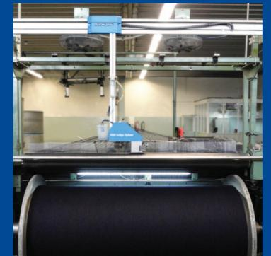
ATS "C" type with JOINTAIR® 115 on flat ATS "L" with INDIGO SPLICER 4662 installed on a **Rebeamer** - downstream of rope dyeing.
