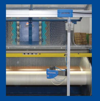
4923B placed in front of a fractional warping weft creel for top-to tail join. machine for cotton yarn.
