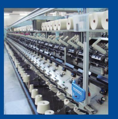
ATS "H" type with HOT JOINTAIR® 4984B on Hank to Cone winder processing worsted and woollen yarns, cashmere and wool blends.
