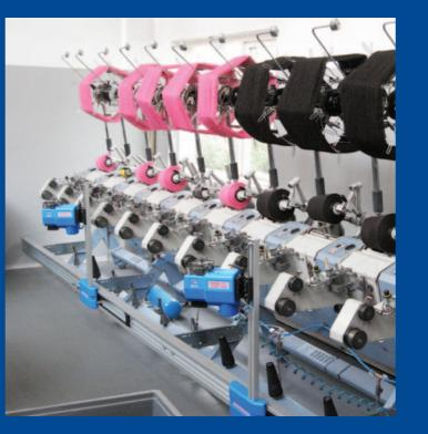
ATS "C" type with floor guide and JOINTAIR® JOINTAIR® 115 fitted in a fixed position 115 fitted on a slider to splice at different level utilising one splicer for two winding heads on hankworsted yarn on reeling machine creel.
