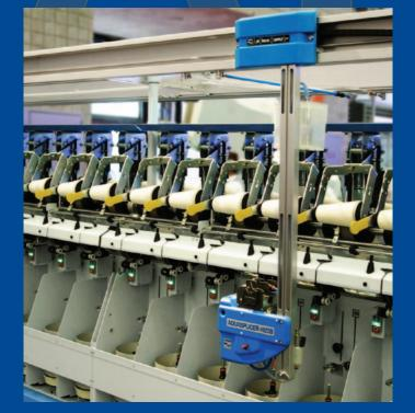
ATS "L" type fitting AQUASPLICER® 4923B instaled **on two-for-one twisting machine** processing fine plied compact cotton yarn.
