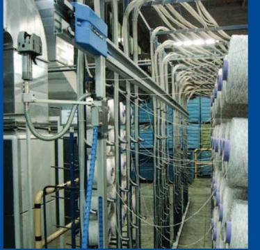
ATS "C" with floor guide fitting JOINTAIR® 116 on a sliding bar with swivel joint enabling splicer vertical movement on the **Tufting creel**.
