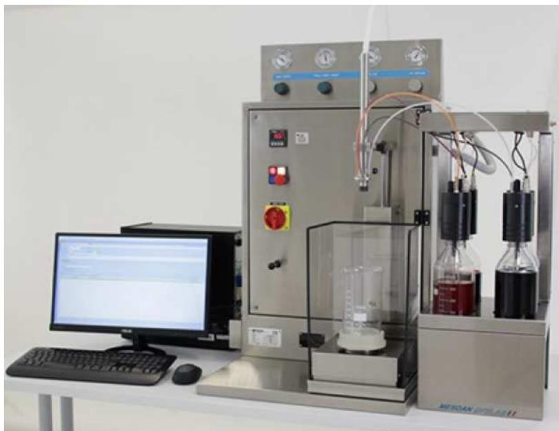
Automatic Dosing System of stock solutions and/or chemical auxiliaries - from max no.4 containers - for colour recipes preparation, (code 323G.140).
